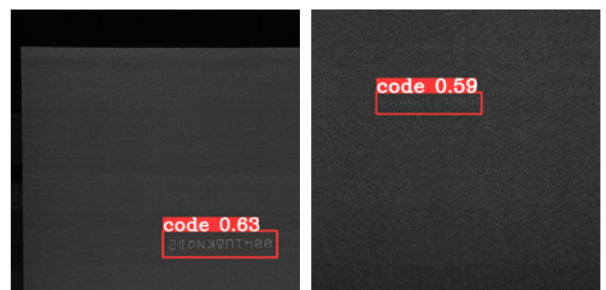
Fig. 1: ROI detection with YOLOv6 model for aluminum (left) and steel (right) plates [3]
