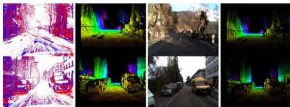
Fig. 3: Demo images of the DSEC dataset with events represented as frame on the left and its disparity ground truth right beside. To the right, RGB frames are shown with their corresponding disparity ground truth. From [4]
