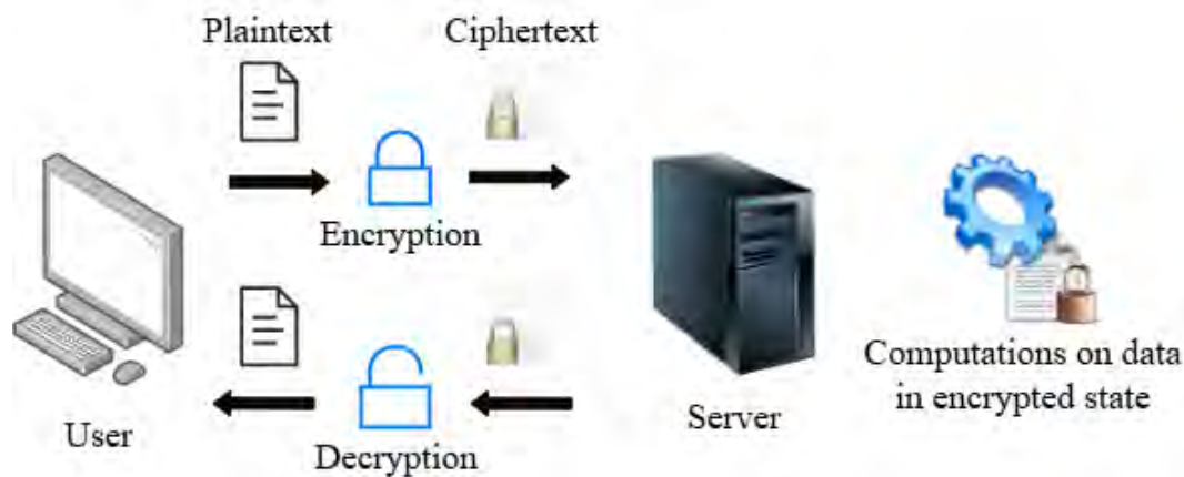
Fig. 1: Processing of homomorphically encrypted data [4]
