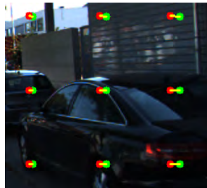
Fig. 6: Re-projected pixels after multiplying the focal length by 0.96 at a focal length of 959px. Small changes in the focal length show a noticeable projection error, the error increases corresponding to the distance of the image center. [4]
